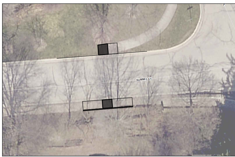
West Crossing of Lane Pl and Summit St: Shift existing ramps approximately 5.0' west; Install B-Curb on south sidewalk edge
