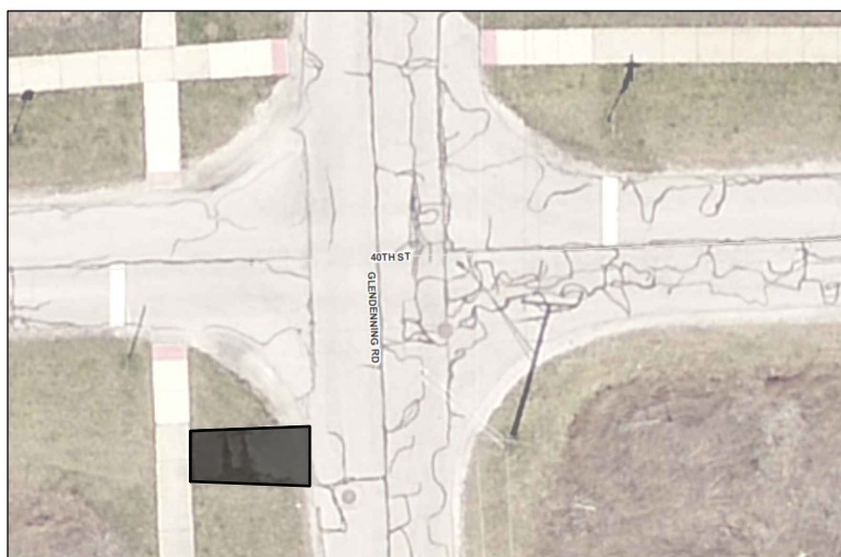
Southwest corner of 40th St and Glendenning Rd: Remove existing HMA pad and restore with topsoil and sod
