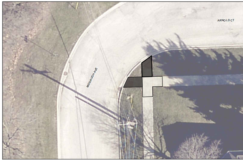
Southeast corner of Middaugh Ave and Arnold Ct: Remove existing sidewalk ramps and restore with topsoil and sod
