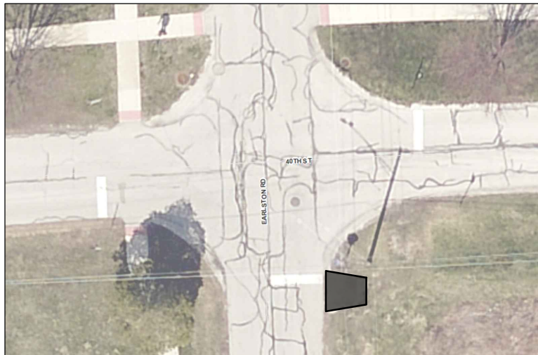
Southeast corner of 40th St and Earlston Rd: Remove existing HMA pad and restore with topsoil and sod
