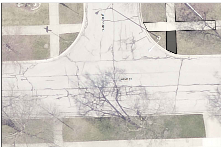
Northeast corner of Plymouth St and 62nd St: Remove existing sidewalk ramp and restore with topsoil and sod
