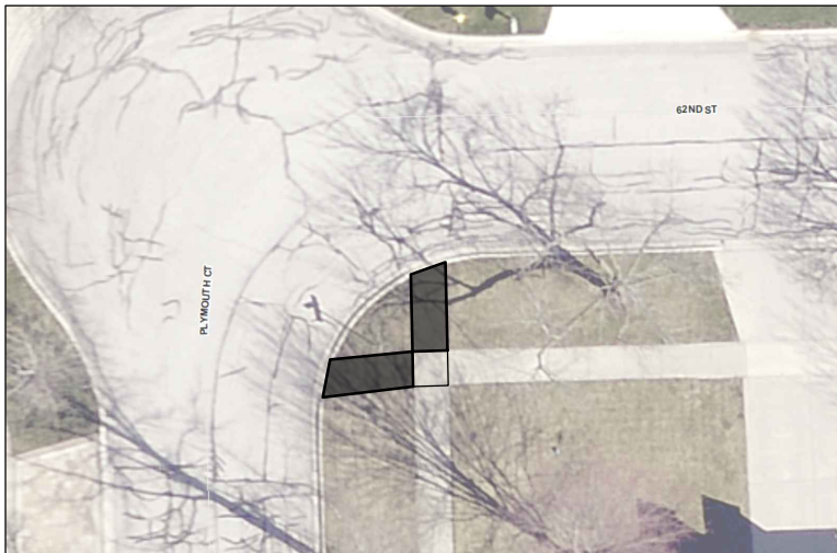
Southeast corner of 62nd St and Plymouth Ct: Remove existing sidewalk ramps and restore with topsoil and sod
