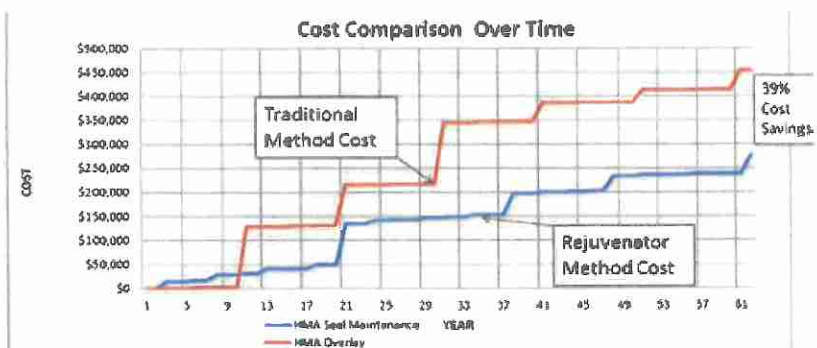
When treatments were averaged out, the resulting graph for partial treatment showed doubling the life of the pavement and savings in excess of 39 percent when compared to conventional roadway mill and resurfacing
