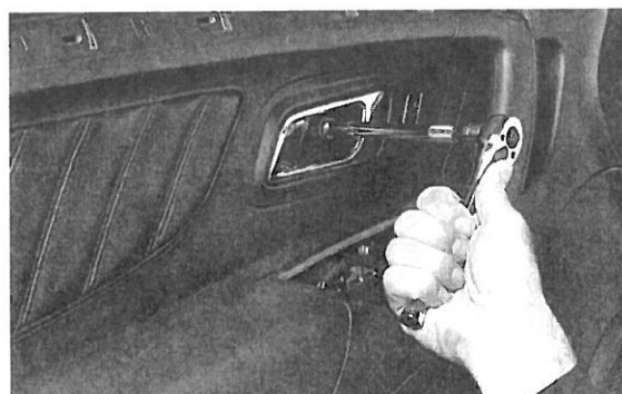
▲ Figure 13. Removing the 10 mm bolt behind the door handle
