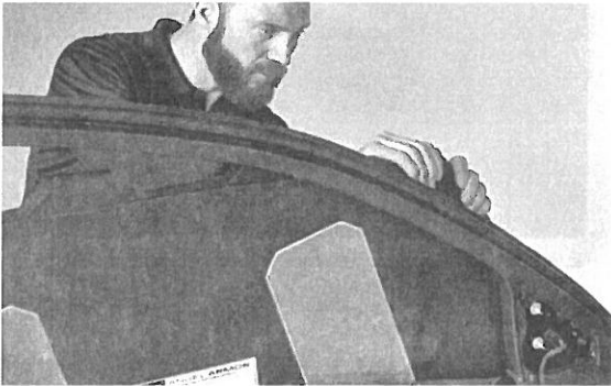
▲ Figure 26. Leaning back while inserting the panel to help avoid obstructions inside the door
