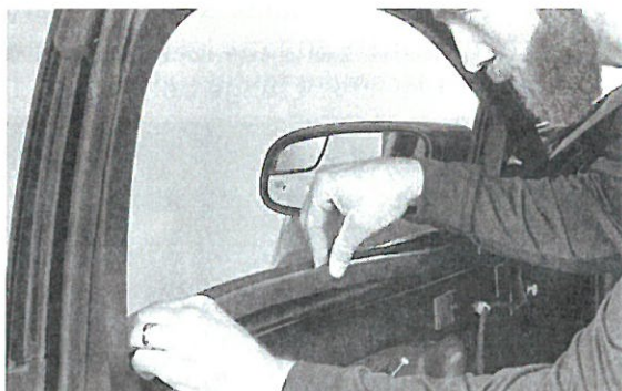
▲ Figure 33: Replacing the interior weatherstrip
