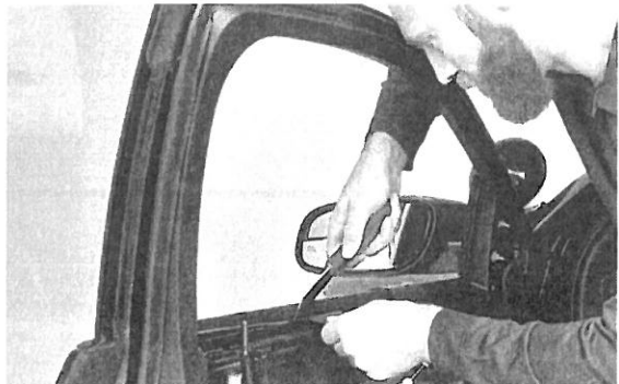
▲ Figure 28. Using the pry tools to push the ballistic panel down and under the outside sheet metal lip
