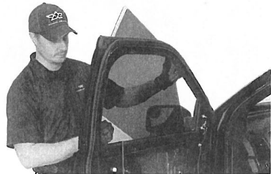
▲ Figure 31. Removing the window glass.
