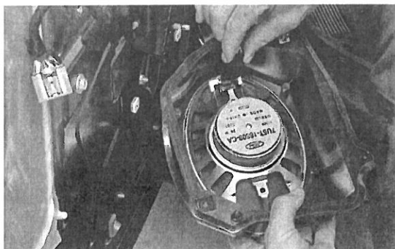
▲ Figure 24. Disconnecting the speaker wiring harness
