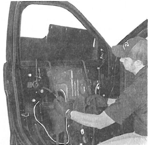
▲ Figure 42. Using the cradle created by the installation straps to lower the armor into the door.
