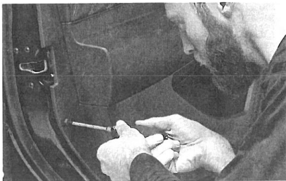
▲ Figure 11. Removing the Phillips screw from the rear end of the door panel
