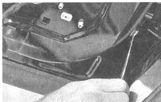
▲ Figure 25. Removing factory installed 13 mm bolt, and replacing it with the supplied hex head bolt.
