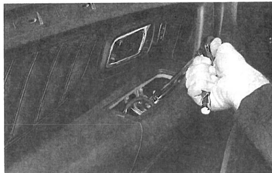
▲ Figure 14. Removing the 10 mm bolt from behind the armrest pocket.
