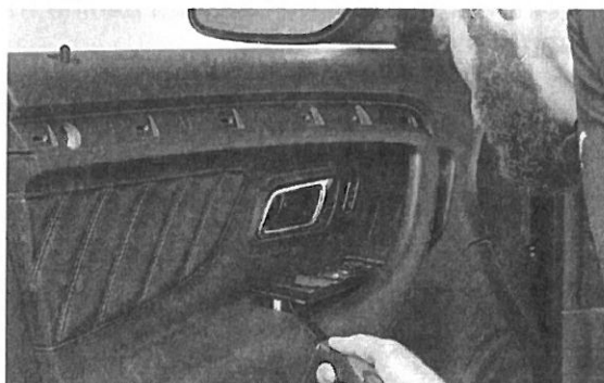
▲ Figure 9. Removing the window control panel
