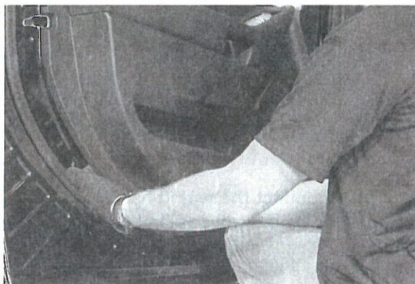
▲ Figure 27. Prying the door panel away from the door skin.
