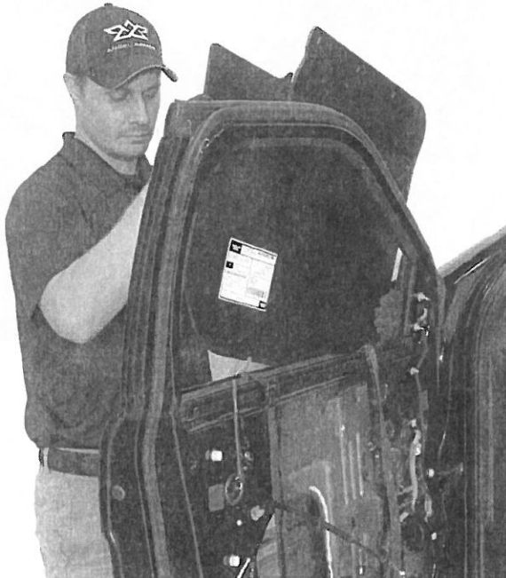
▲ Figure 41. Placing the armor into the door.
