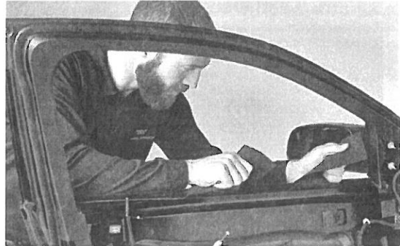
▲ Figure 27. Gripping ballistic door panel's top-edge nylon folds and sliding the panel forward
