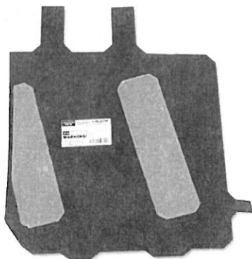
▲ Figure 2. Angel Armor Avail Ballistic Door Panel (Level IIIA) for Ford Police Interceptor Sedan
