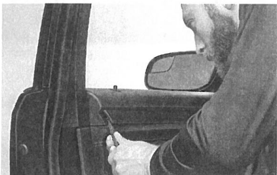
▲ Figure 7. Removing the trim above the door handle
