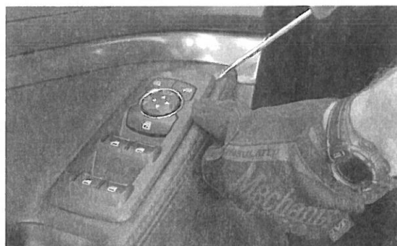
▲ Figure 25. Prying up the window control panel.
