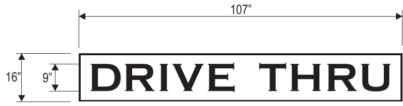
D/T WALL SIGN ELEVATION: 3/8" = 1'-0" 11.89 SQ.FT.
