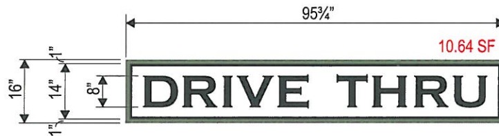
D/T WALL SIGN ELEVATION: 3/8" = 1'-0"
