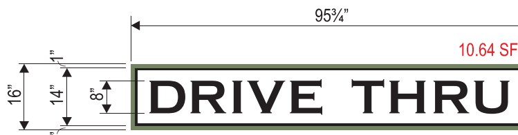
D/T WALL SIGN ELEVATION: 3/8" = 1'-0"
