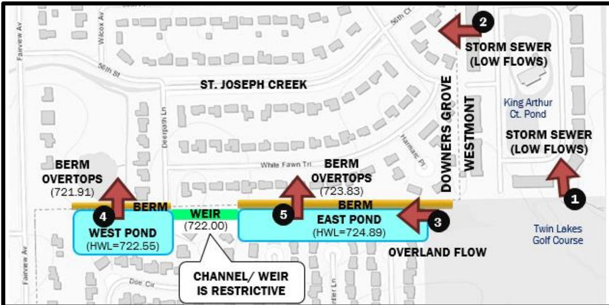
**Figure 4:** The existing stormwater runoff conditions through the subdivision are depicted with arrows. During large storm events, high flows fill the ponds and stormwater overtops the berms.
