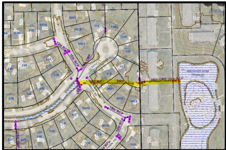
**Figure 5:** Highlighted pipe shows location of undersized storm sewer from King Arthur Court Apartment pond to St. Joseph Creek.
